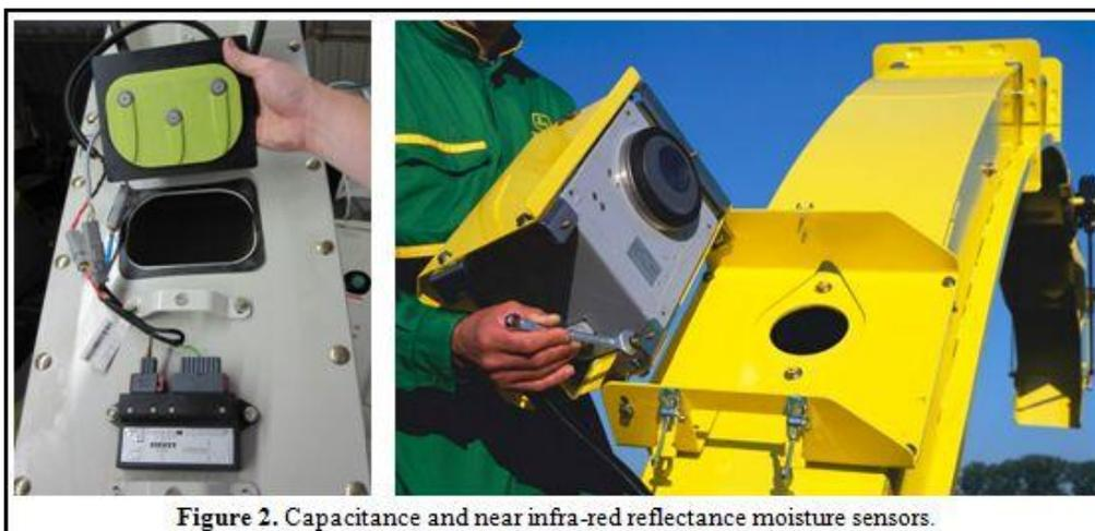
Figure 2. Capacitance and near infra-red reflectance moisture sensors.
