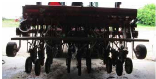
Figure 1. Modified grain drill to allow seeding into corn.
