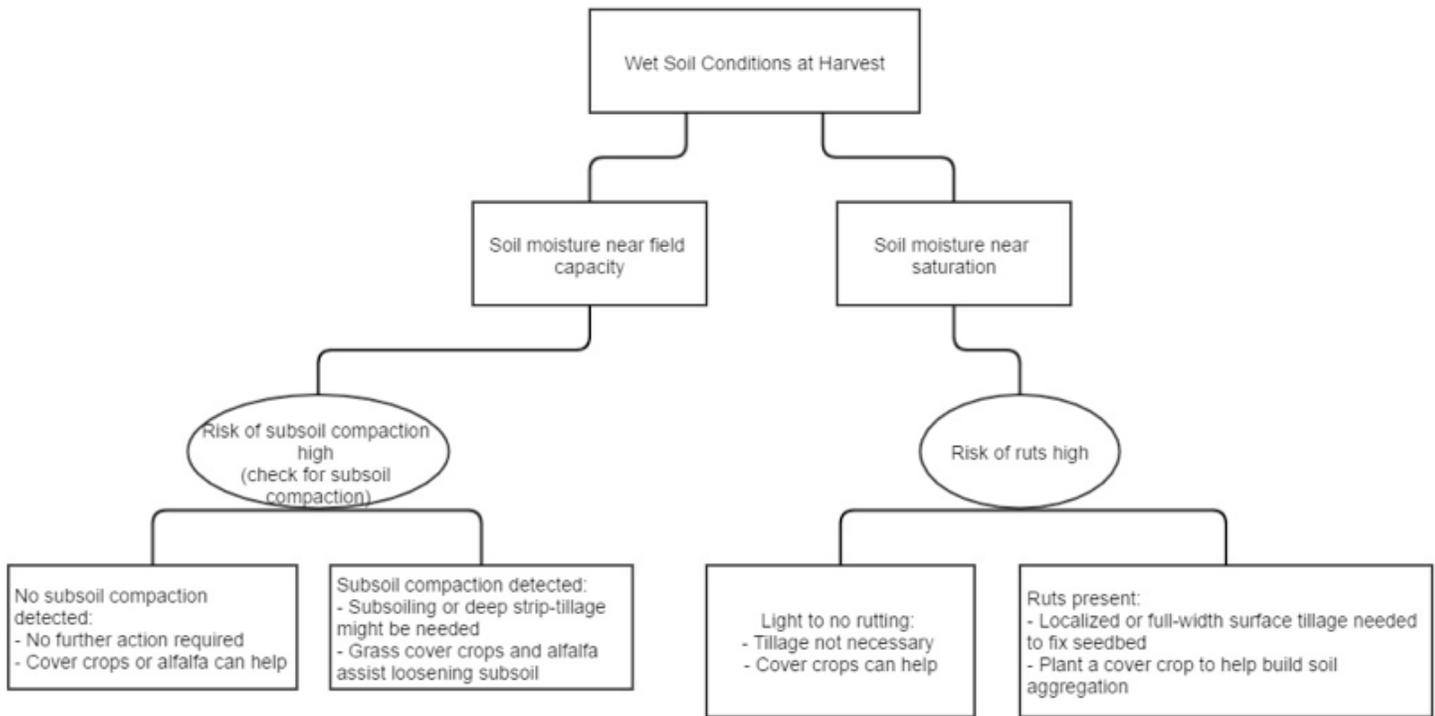
**Figure 2.** Decision diagram to assist in determining soil compaction presence after harvest during wet field conditions.
