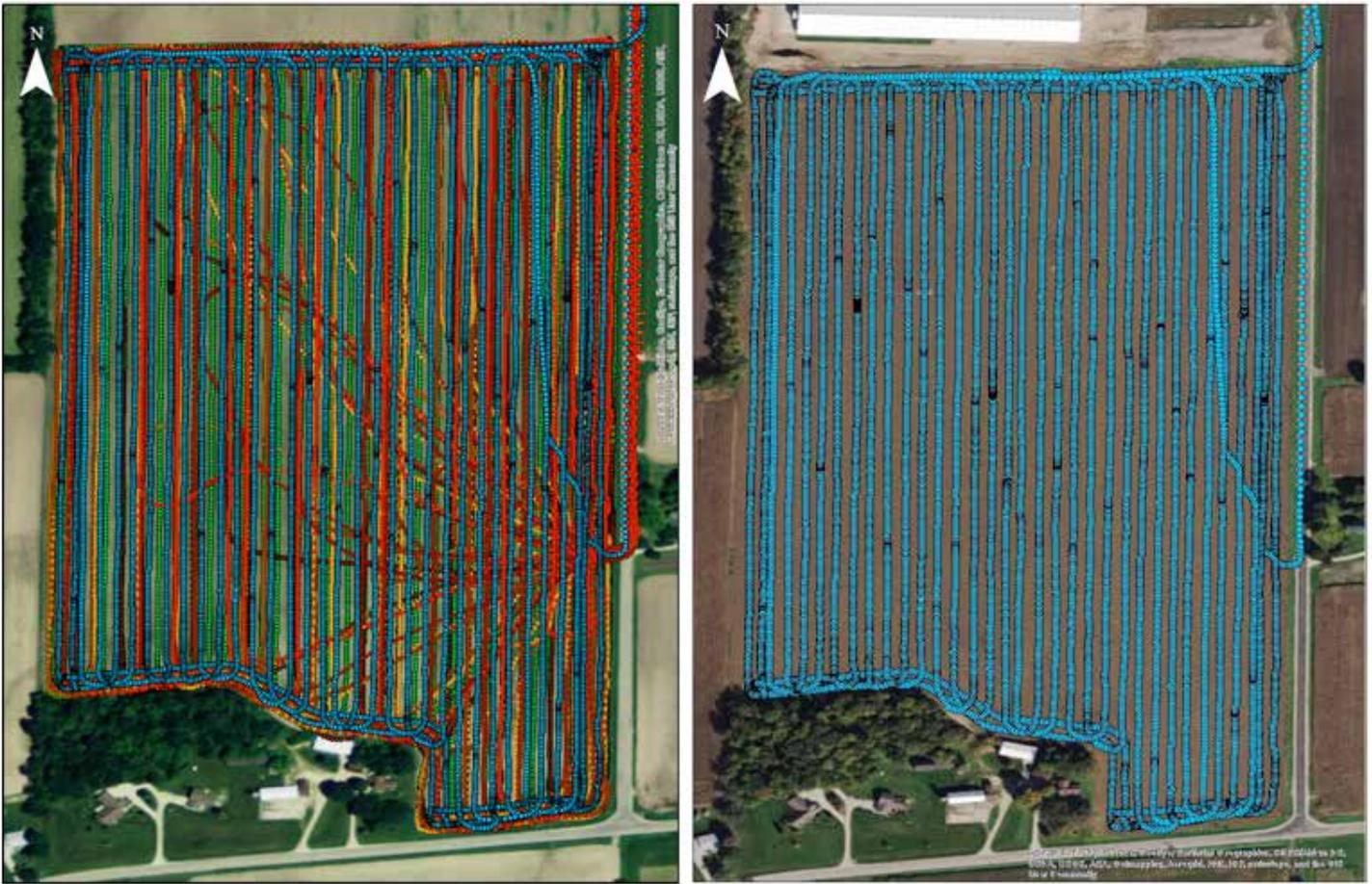
**Figure 1.** Global positioning system data of an alfalfa forage harvest operation with all equipment involved; merger path, chopper path, and six transport trucks **(Left)**. Global positioning system data of forage harvester path only simulating controlled traffic within a harvest operation **(Right)**.
